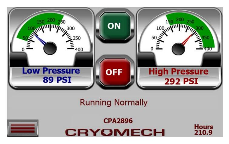
The "Home" screen is the default starting up screen. It is assumed that most facilities will have this screen up and running over the life of the compressor. The left dial indicates the low or gas input pressure and the right dial indicates the high or output pressure. Status about the running state of the compressor will be displayed on the Feedback Label. The bottom right Hours number tracks the total hours of operation the compressor has been running.
