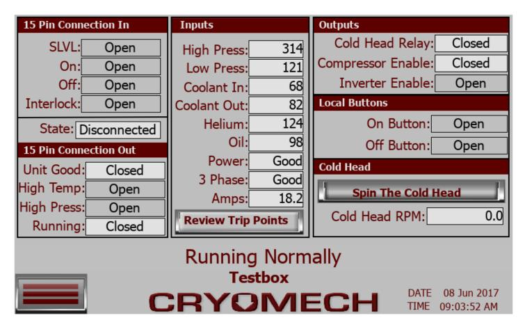
The diagnostics screen is used to indicate the status of the different digital inputs and outputs. This screen is useful for diagnosing running issues if they arise. If you click on the Review Trip Points button the next screen will appear allowing the operator to review what temperatures and pressures this system will alarm at.
