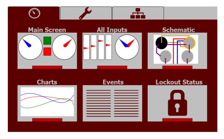
This screen allows the operator to navigate between various status screens or to adjacent menu screens.
