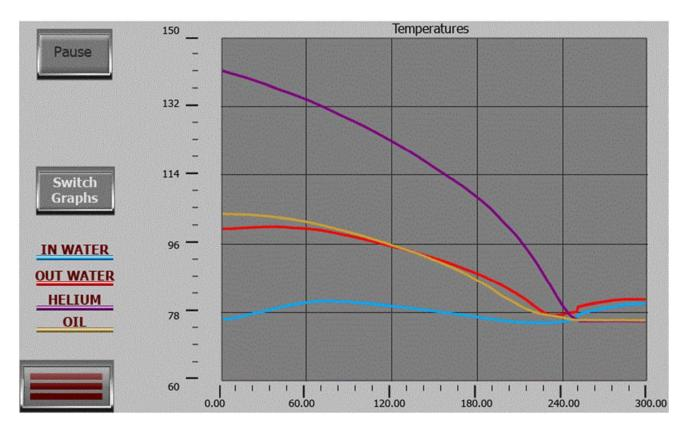
The charts screen has two modes. One is the temps reading mode and the alternate is pressure monitoring. When the temps mode is selected the time span is 5 minutes. Temp data is collected in 1 second intervals and is displayed with the newest data on the right hand side of the chart. The scales will auto adjust based on the data displayed.
