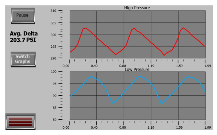
The pressure monitoring mode has a time span of 2 seconds. The high and low pressures scales are independent and auto adjust based on captured data. A pause button is provided to allow closer examination of the charts.
