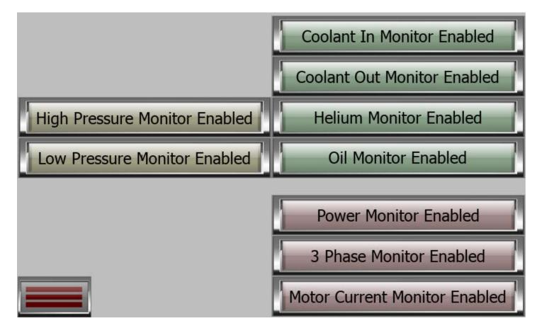
This screen allows the operator to disable a single sensor, the sensor may be ignored allowing the compressor to run until such time that the sensor can be replaced.
