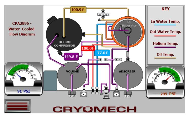
The "Schematic" screen is designed to give the general idea of how all the components are connected. It also indicates the current temperature readings for the various parts of the system. To the left and right of the schematic are the "Low" or Inlet and "High" or outlet pressures.
