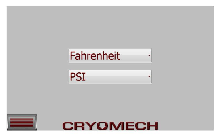
The "Unit of Measures" screen is used to set what sorts of units we wish to display on the screen. For temperature, you can select between Celsius, Fahrenheit or Kelvin. For pressure, you can select between PSI, BAR & KPSA. Selecting here will affect most other screens.
